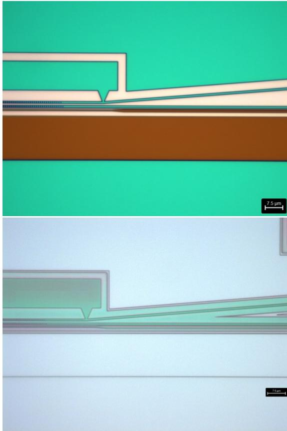
Figure 4- Sleeve for EBL with the bulk etched afterwards.
