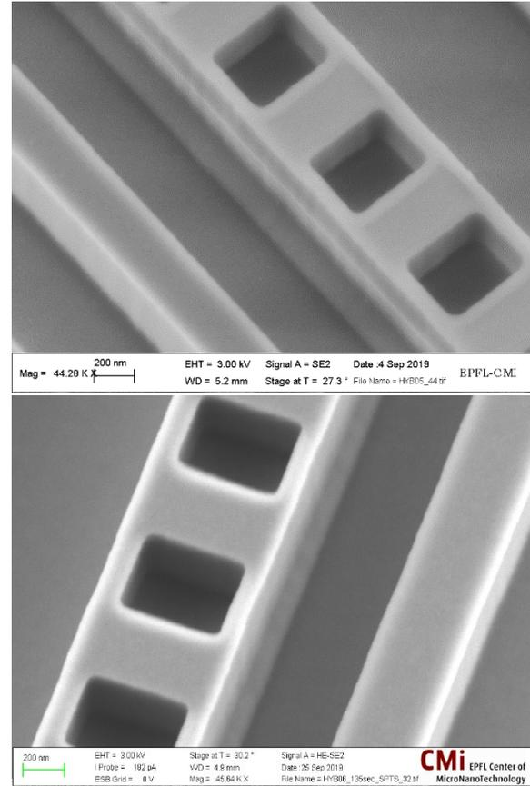
Figure 5- Top shows the conventional compared to bottom one using the bulk and sleeve method.
