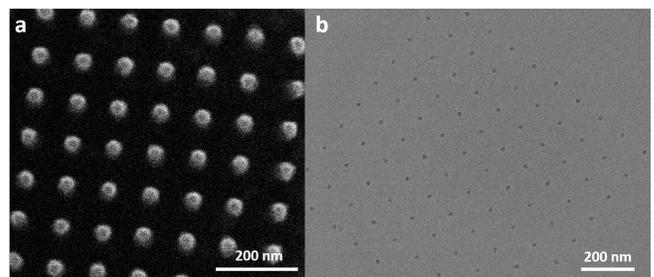
Figure 3. **Aluminum nanodisks fabricated on a 5-nm-thick SiN membrane.** (a) SEM image of an array of nanodisks with a large diameter created with a high exposure dose. (b) Bright-field TEM image of an array of nanodisks with a small diameter created with a low exposure dose.
